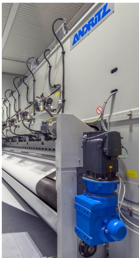
Needleloom with integrated Zeta drafter
